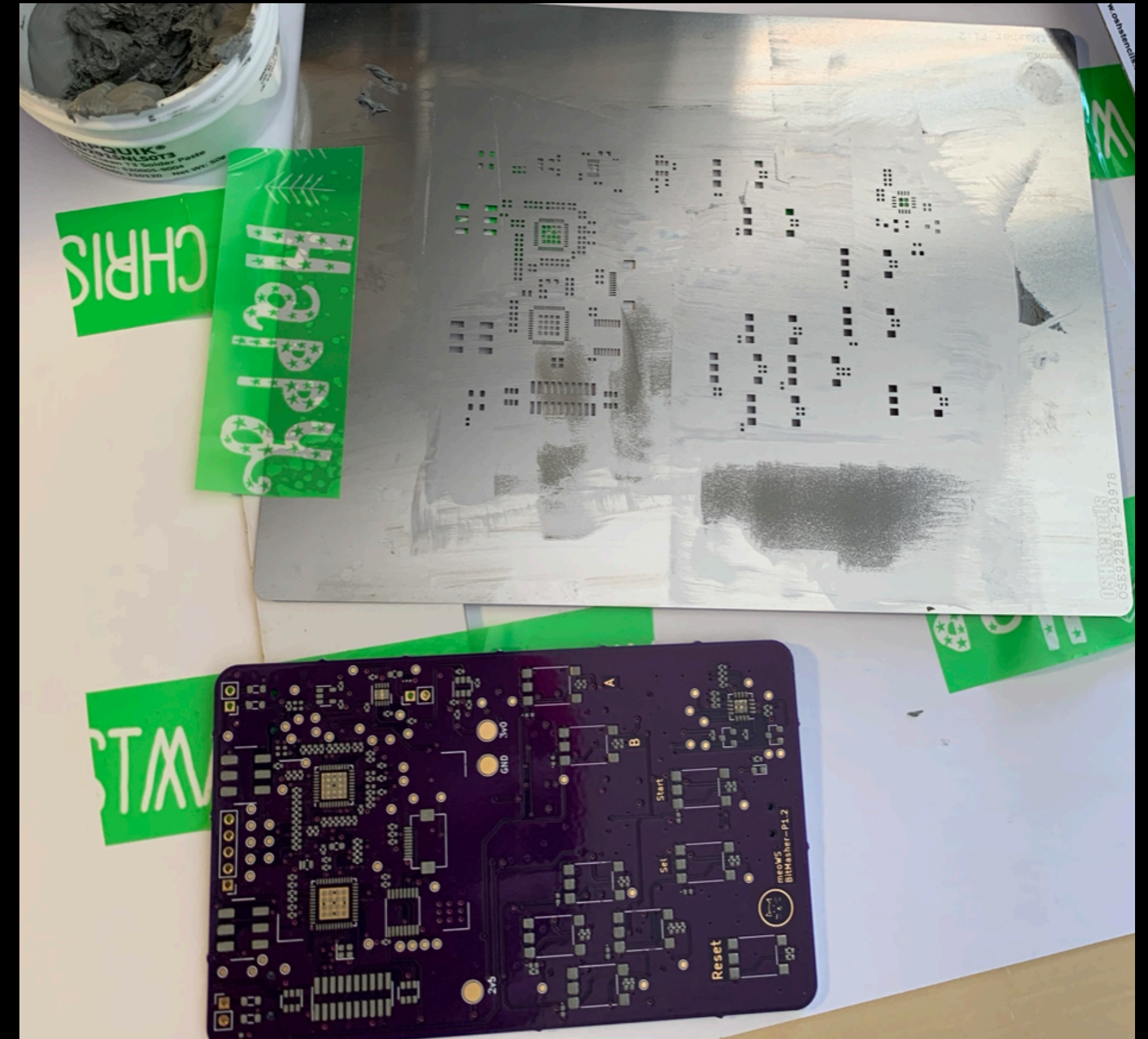
Preparing PCB for Reflow
